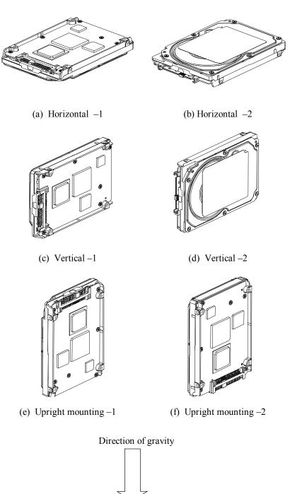
Figure 4.2 HDD orientations
